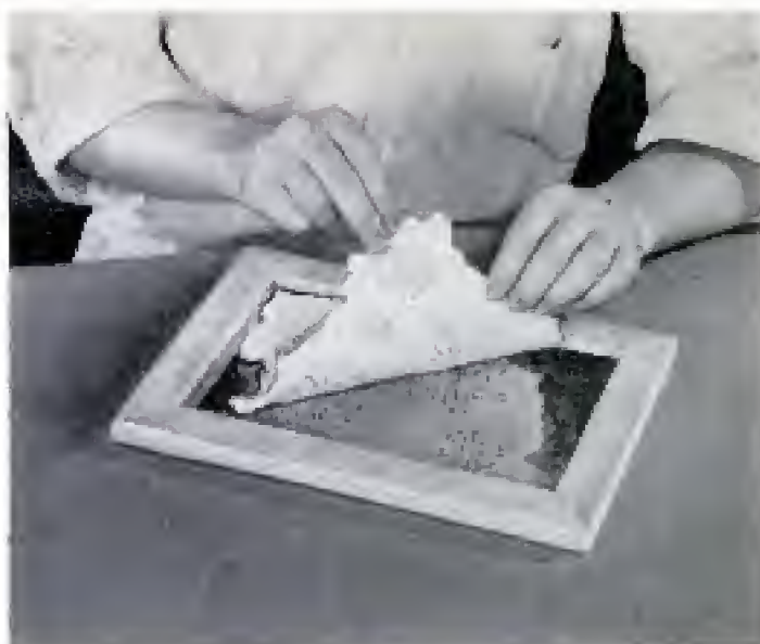
After the liquid rubber has set, above, it is pulled away from the beeswax mold. All wax is cleaned from the plate
